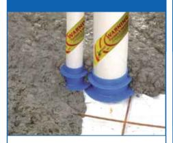
HomeGuard Collars are innovative, preformed rigid collars which are designed to prevent concealed termite entry via penetrations. They are manufactured from polyethylene, impregnated with Biflex termiticide, which repels and kills termites on contact preventing ingress via the sub soil.
