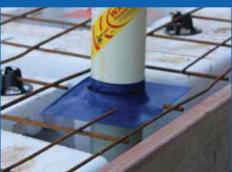
HomeGuard FlexiCollars are a innovative, preformed single layer collar which are designed to prevent concealed termite entry via penetrations. They are manufactured from plastic that has been impregnated with Biflex termiticide, which repels and kills termites on contact preventing ingress via the sub soil.
